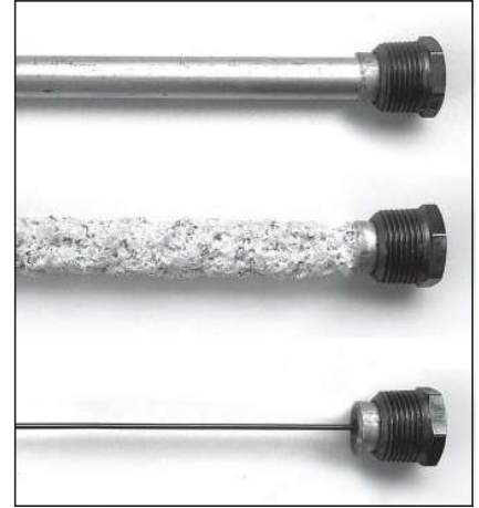
Figure 40 - Anode rods from new (top) to partially depleted (middle) to fully depleted stage (bottom).
